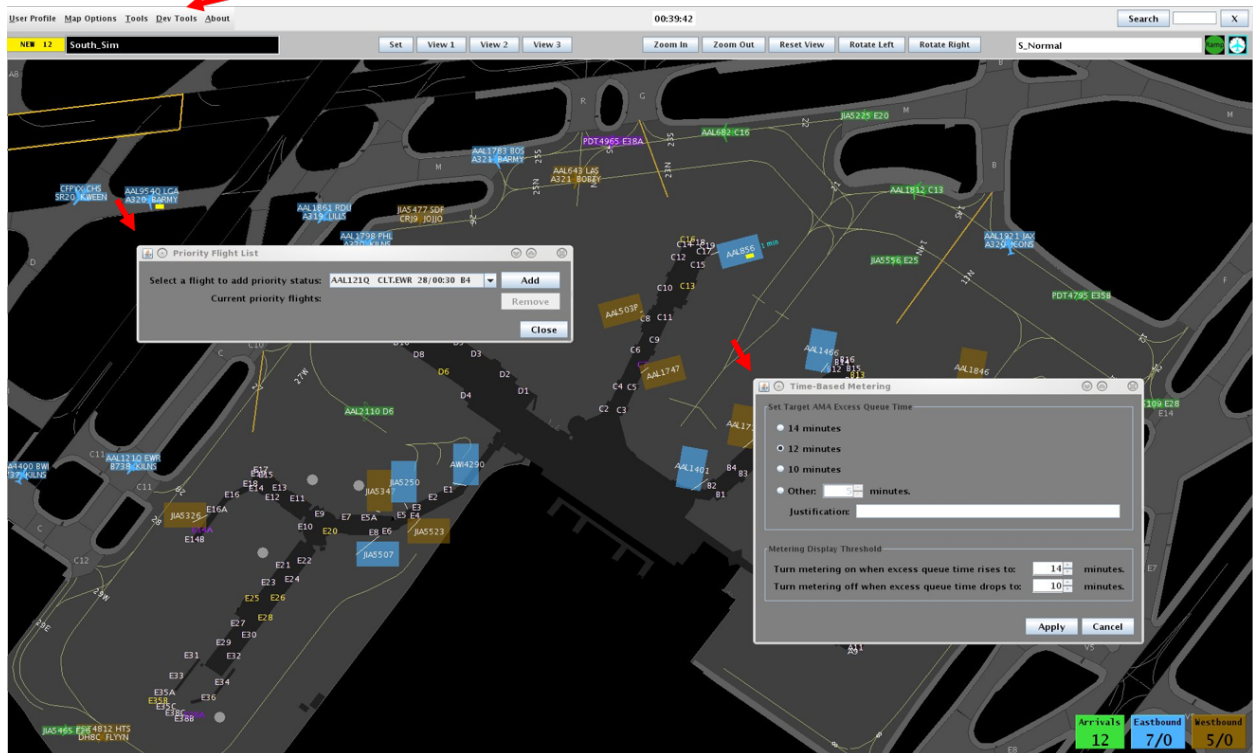
Figure 20 - The Ramp Manager Traffic Console (RMTC) display provides many functions and capabilities in an automated format to the Ramp Manager through multiple feature windows.
